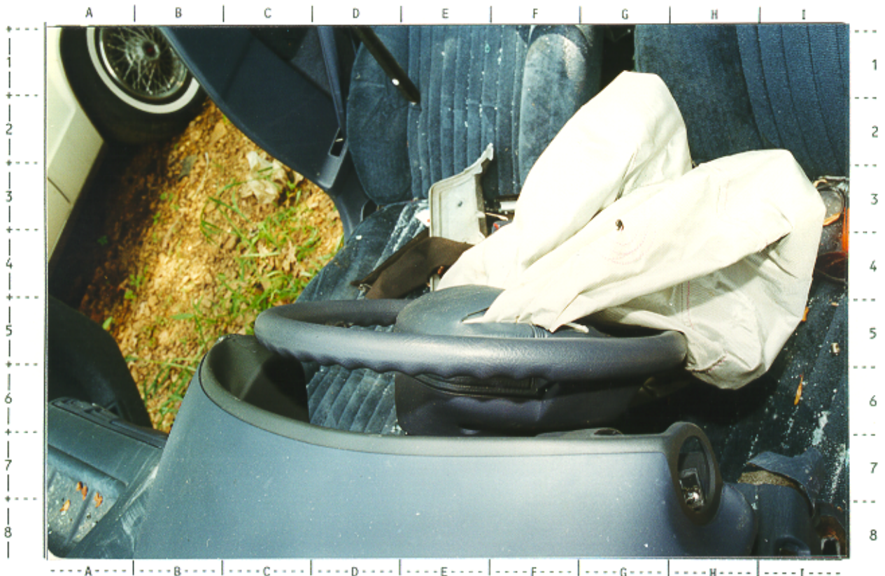
# 52 -- Overhead left center view of 1991 Chevrolet Corsica's undeformed steering wheel and deployed air bag
